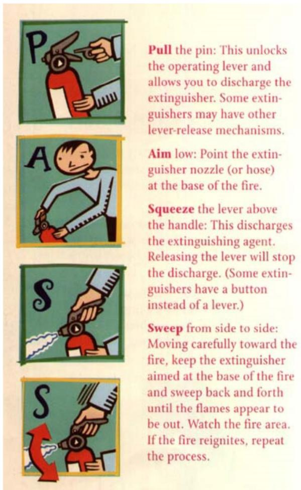
**NOTE:** Never attempt to use a fire extinguisher to extinguish a large or rapidly spreading fire. Never re-hang a spent fire extinguisher back on the wall.
